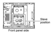
Attaching the external disc unit to the DVR
